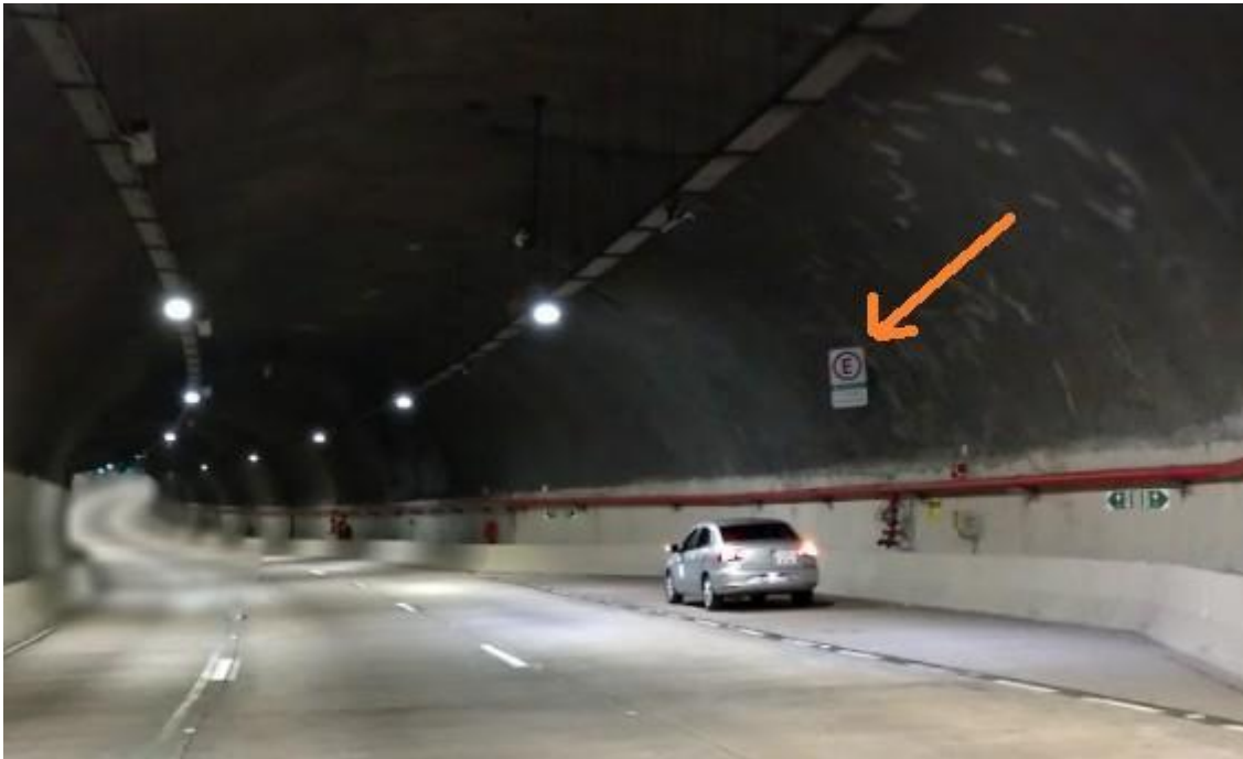
Figure 11: Signpost in the pull-off, seen from a distance, giving the impression that parking is allowed
